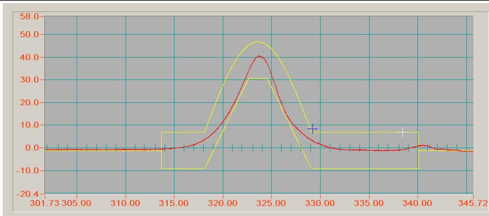
The curve of Shock test (+Y axis)
