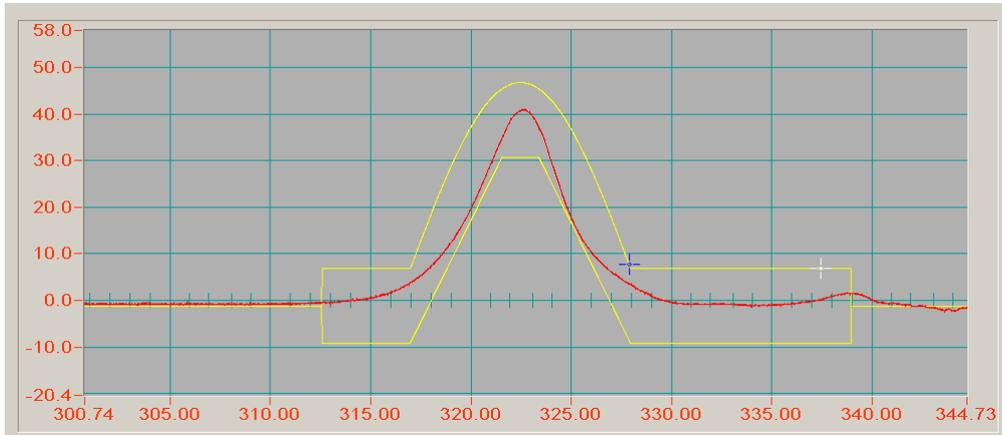
The curve of Shock test (+X axis)
