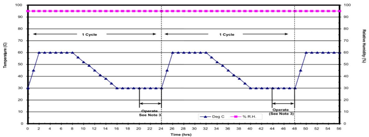
**Figure 507.5-7. Aggravated temperature-humidity cycle.**
