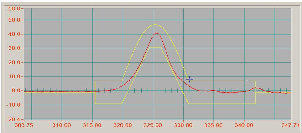
The curve of Shock test (-Y axis)
