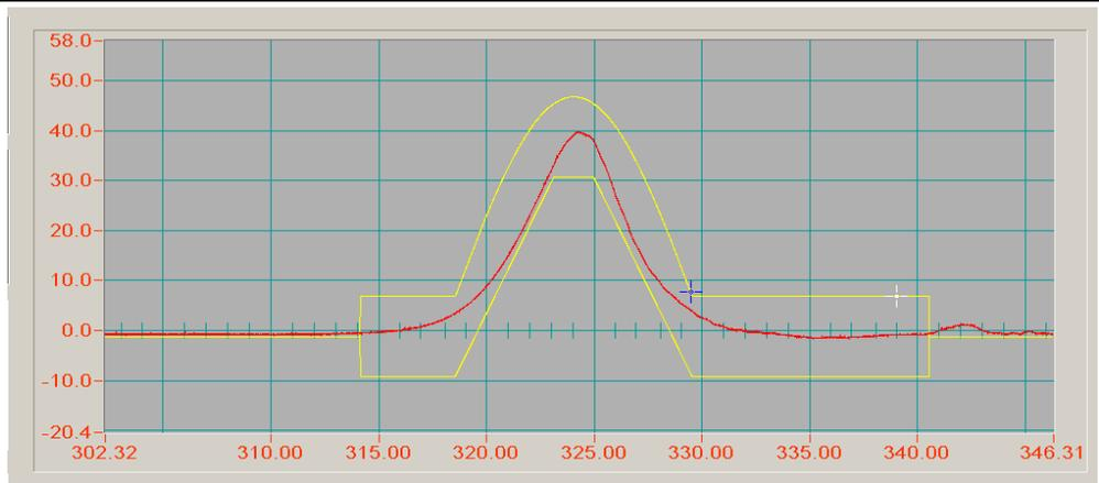
The curve of Shock test (-Z axis)
