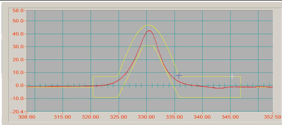
The curve of Shock test (-X axis)
